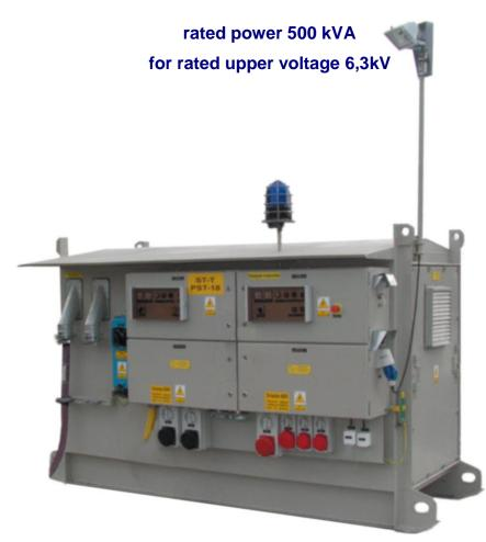
The transformer station type ST-T is a device designed for use on the ground with no explosion hazard. The transformer station ST-T is equipped with a power protections against short-circuits, overloads and lowered insulation resistance (for 500V AC) with installed three-core transformer: 500 (400+100) kVA and lower rated voltage of transformer 500V AC (for 400 kVA) i 400V AC (for 100 kVA).
